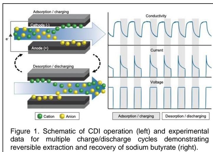
**Electrically driven ion adsorption and recovery was demonstrated for butyrate, a key input for bio-based hydrocarbon fuels and chemicals.**
