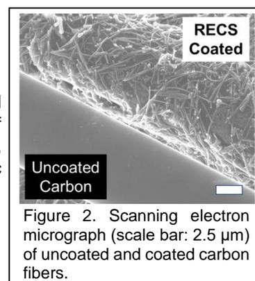
Figure 2. Scanning electron micrograph (scale bar: 2.5 μm) of uncoated and coated carbon fibers.
