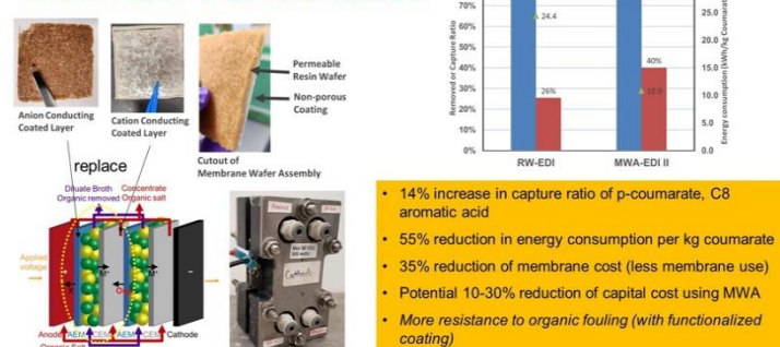
Figure 2. Comparison of separation performance by RW-EDI and MWA-EDI technologies.
