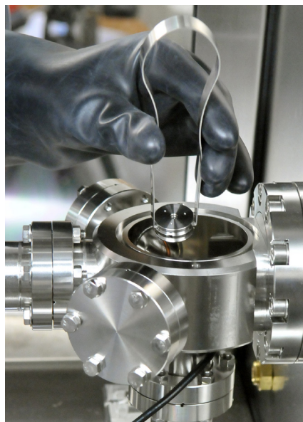
Loading a sample into the antechamber of the XPS.
