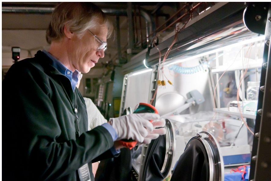
Argonne scientist Ira Bloom prepares to open a lithium-ion cell. Prior to opening the cell, a thermocouple is attached to provide information on cell temperature.
