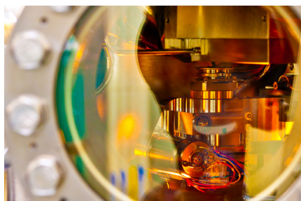
A view of the heart of the X-ray photoelectron spectrometer unit, showing the servo-motor and the stage that it moves.
