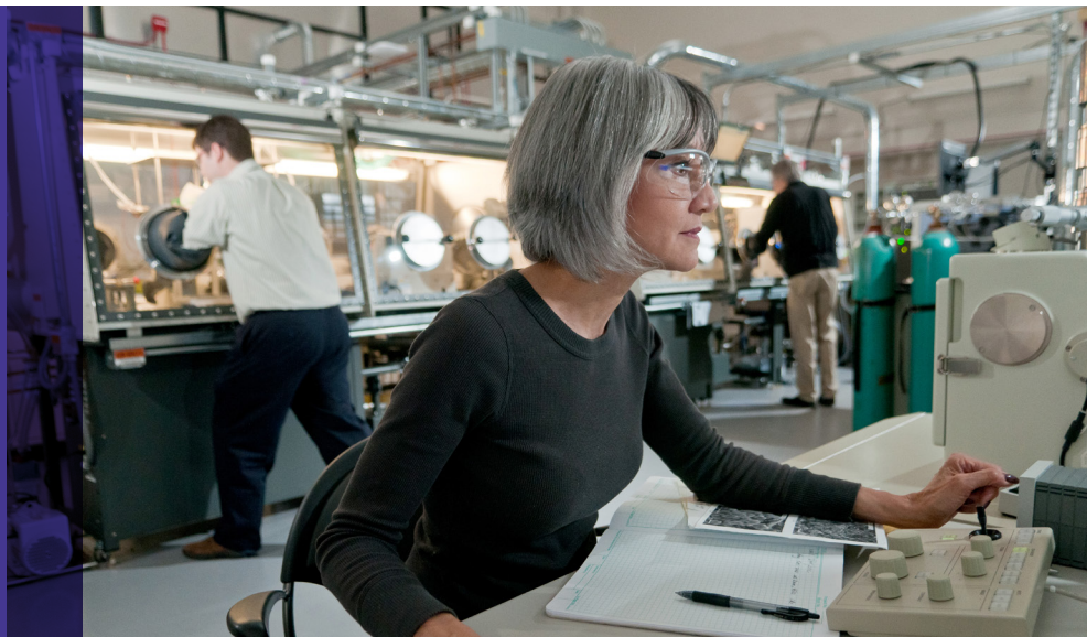
Argonne scientist Nancy Dietz Rago analyzes results in the Post-Test Facility. After a battery sample is characterized in the large glove box, it is transferred without exposure to air to the scanning electron microscope for detailed, microstructure characterization.
