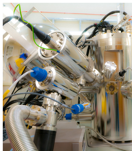
An X-ray photoelectron spectrometer (XPS) is integrated into the Post-Test Facility's large, central glove box. The XPS is used to determine the chemical environments present on the surface of a material.
