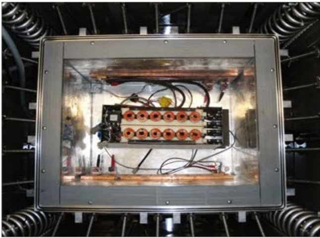
A large battery module in the Large-Volume IBC test chamber, with cooling/heating coils in each corner.
